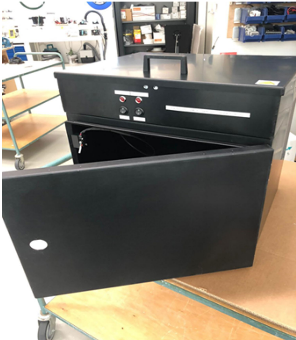
Figure 2. Prototype UV-C test apparatus.
